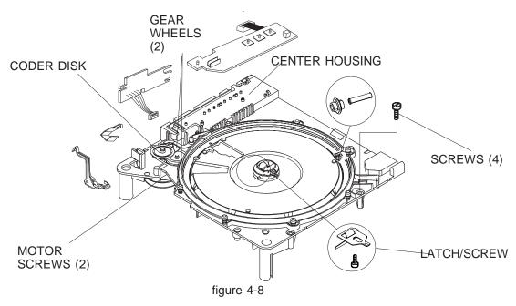
**14**. During disassembly and assembly of the CENTER HOUSING, place the TRAY RELEASE LEVER into the position as shown below.
